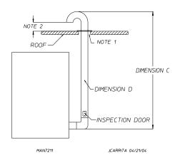
NOTE 1 Opening from combustible materials must be 2-inches (5.08 cm) larger than the duct (all the way around). The duct must be centered within this opening.
